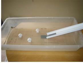
Figure 4. Placement of model houses in flood plain at the base of the landslide chute.
