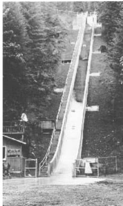
A 100-meter long debris chute used to simulate landslides.
